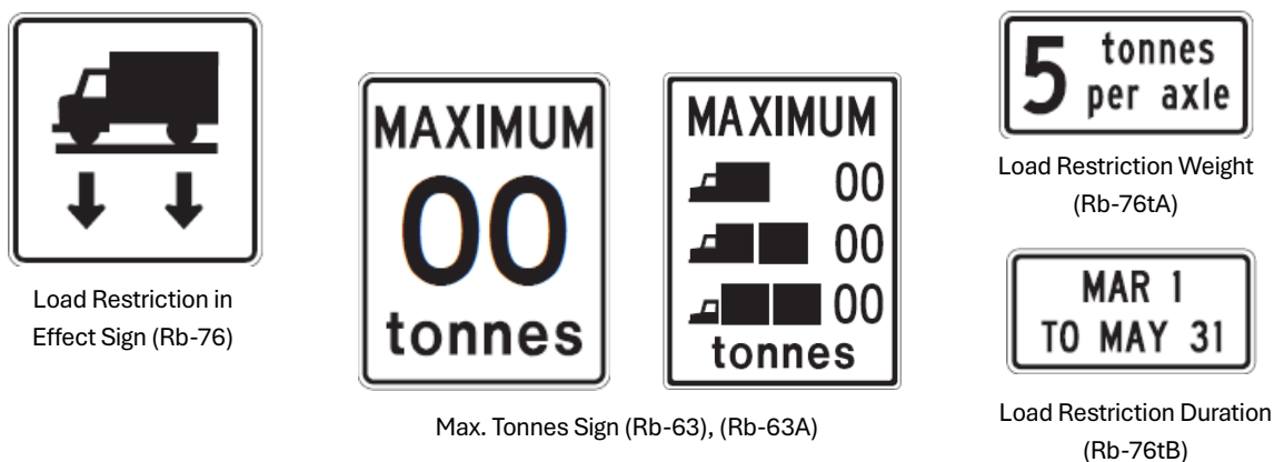
Figure 2: Load Restrictive Signage
